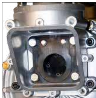
Only 4 bolts to access flap valves
